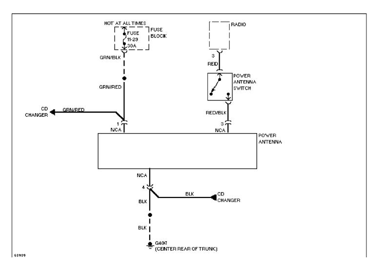
SYSTEM WIRING DIAGRAMS Power Distribution Circuit (1 of 5)
