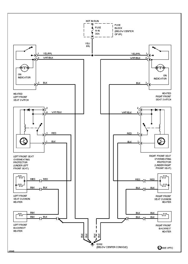
SYSTEM WIRING DIAGRAMS Power Seats Circuit
