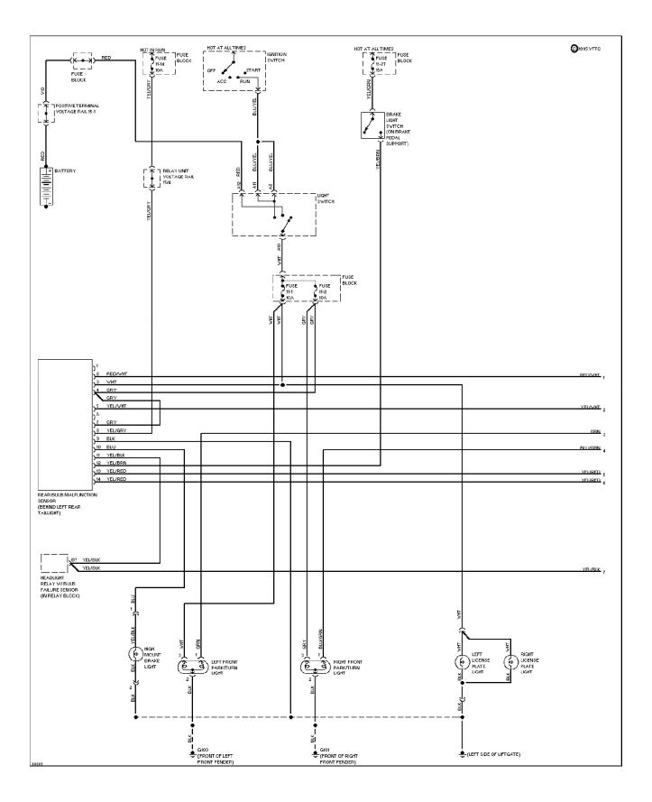
SYSTEM WIRING DIAGRAMS Exterior Lamps Circuit, Wagon (2 of 2) 1994 Volvo 960
