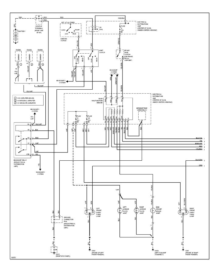
SYSTEM WIRING DIAGRAMS Exterior Lamps Circuit, Wagon (2 of 2) 1995 Volvo 940
