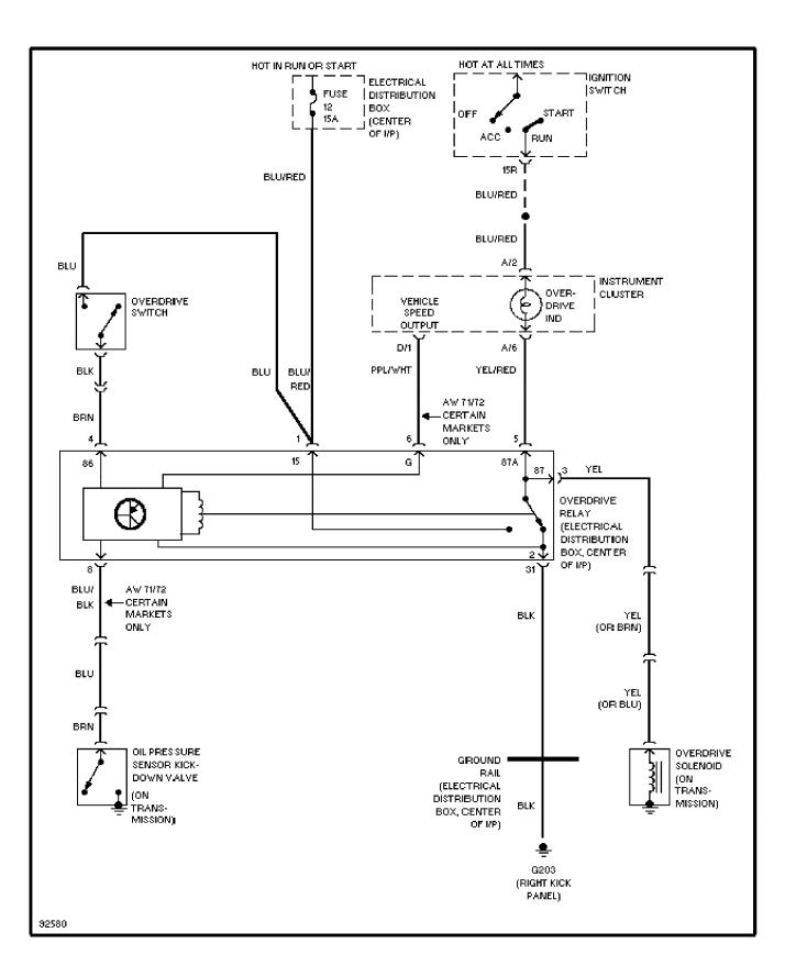
SYSTEM WIRING DIAGRAMS Warning System Circuits 1995 Volvo 940
