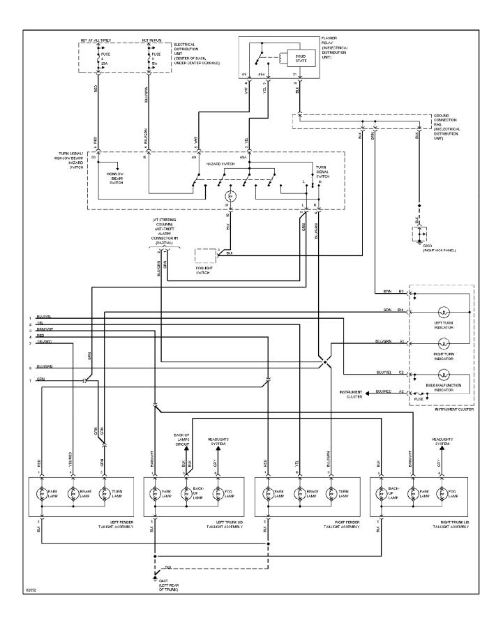
SYSTEM WIRING DIAGRAMS Exterior Lamps Circuit, Wagon (1 of 2)
