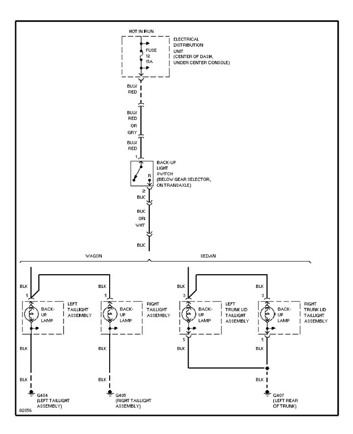
SYSTEM WIRING DIAGRAMS Exterior Lamps Circuit, Sedan (1 of 2)
