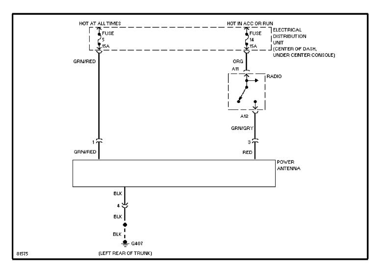
SYSTEM WIRING DIAGRAMS Power Distribution Circuit (1 of 2)
