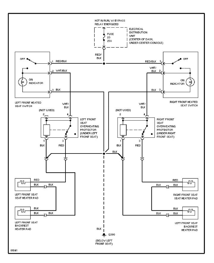
SYSTEM WIRING DIAGRAMS Heated Seats Circuit, Normal Output
