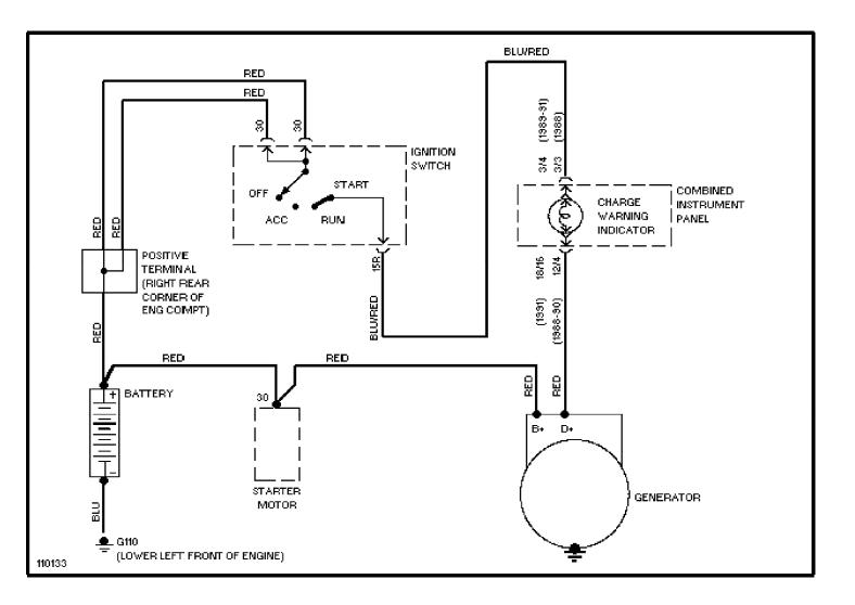
SYSTEM WIRING DIAGRAMS Starting Circuit
