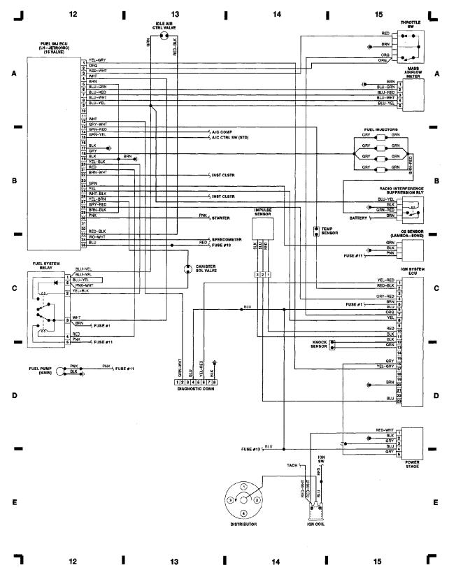
WIRING DIAGRAMS Fig. 5: Computer Engine Control (LH-Jetronic, Turbo) 1989 Volvo 740
