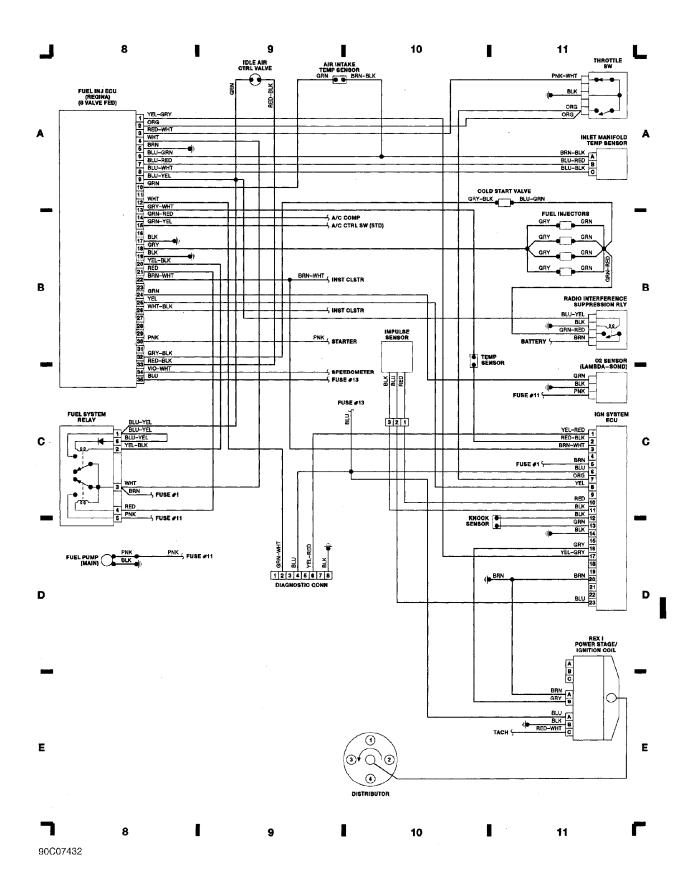
WIRING DIAGRAMS Fig. 4: Computer Engine Control (LH-Jetronic, 16 Valve) 1989 Volvo 740
