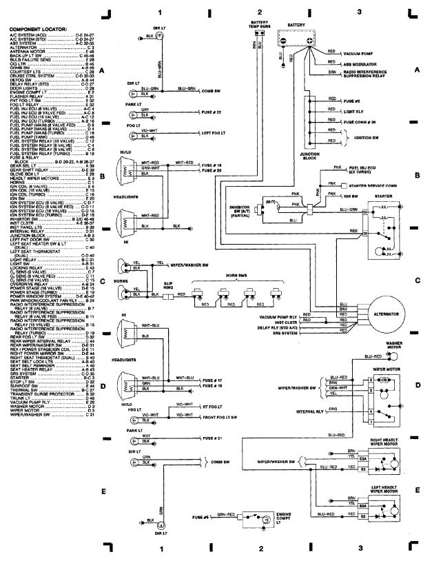
WIRING DIAGRAMS Fig. 2: Computer Engine Control (LH-Jetronic, 8 Valve) 1989 Volvo 740
