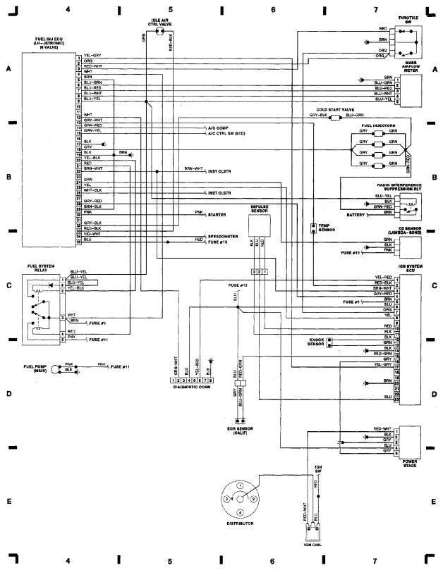
WIRING DIAGRAMS Fig. 3: Computer Engine Control (Regina, 8 Valve) 1989 Volvo 740
