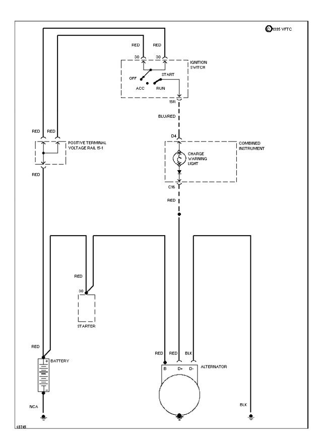
SYSTEM WIRING DIAGRAMS Starting Circuit
