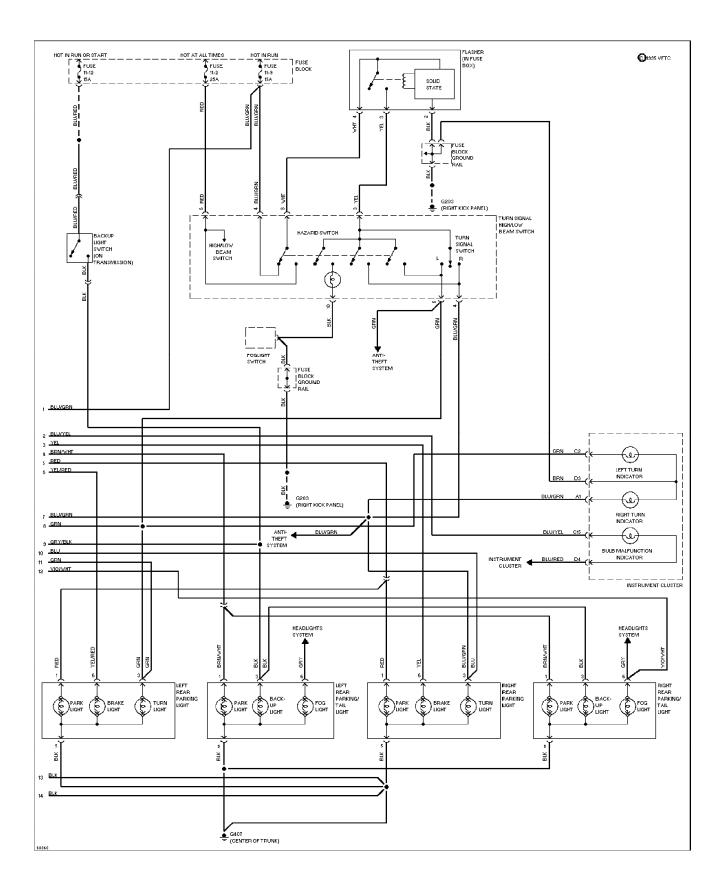
SYSTEM WIRING DIAGRAMS Exterior Lamps Circuit, Wagon (1 of 2) 1994 Volvo 940
