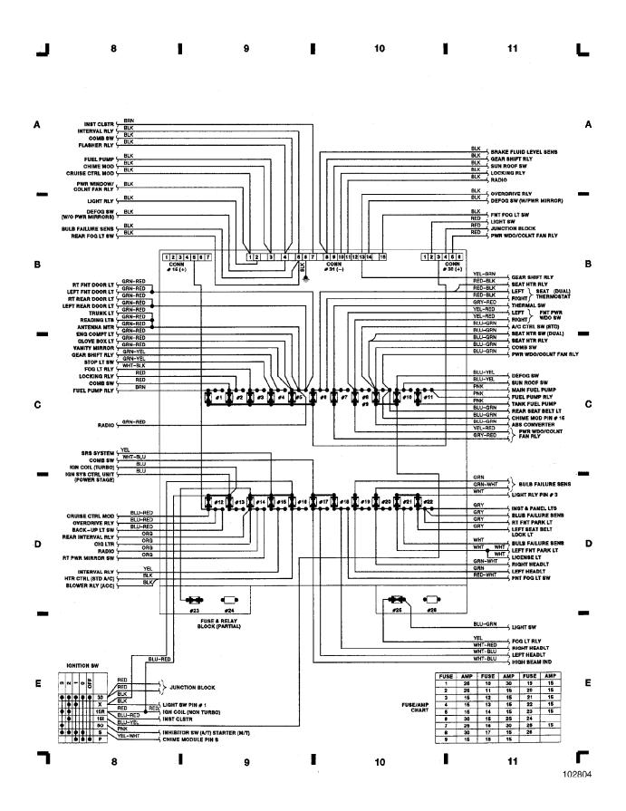
WIRING DIAGRAMS Fig. 4: Relays, Underdash & A/C & Heating 1988 Volvo 740
