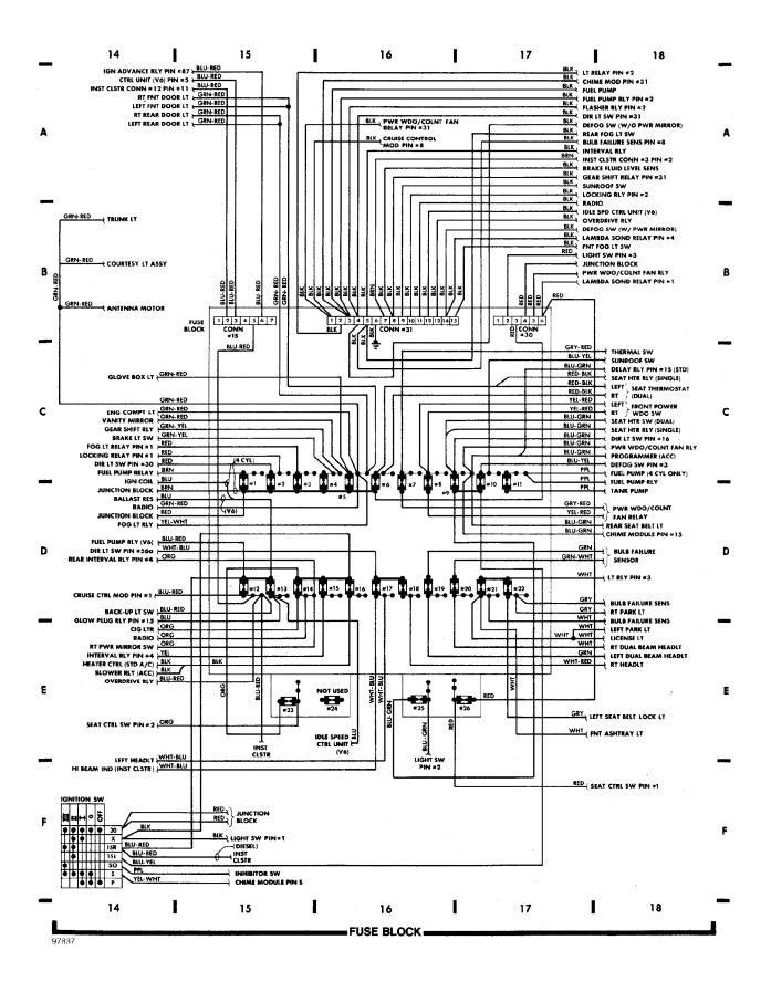
WIRING DIAGRAMS Fig. 5: Underdash (Grids 18-23)
