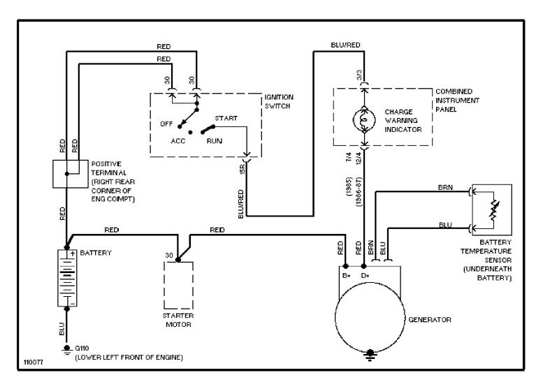
WIRING DIAGRAMS Fig. 6: Underdash (Cont.) (Grids 23-28) 1986 Volvo 740
