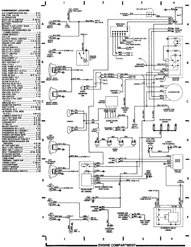
WIRING DIAGRAMS Fig. 2: Engine Compartment (Cont.) (Grids 4-9) 1986 Volvo 740
