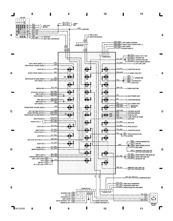
Fig. 4: ECC Control Unit, A/T Control Unit (Grid 12-15) 1993 Volvo 960
