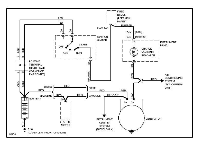
SYSTEM WIRING DIAGRAMS Starting Circuit
