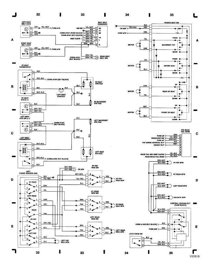
WIRING DIAGRAMS Fig. 10: Passenger Compartment (Cont.) & Taillights 1988 Volvo 760
