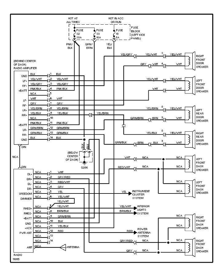
WIRING DIAGRAMS Fig. 7: Anti-Lock Brake System, Cruise Control & Accessories 1988 Volvo 760
