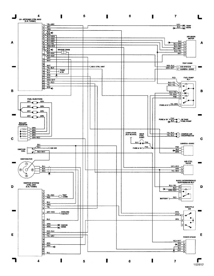
WIRING DIAGRAMS Fig. 3: Computer Engine Control (2.8L V6) 1988 Volvo 760
