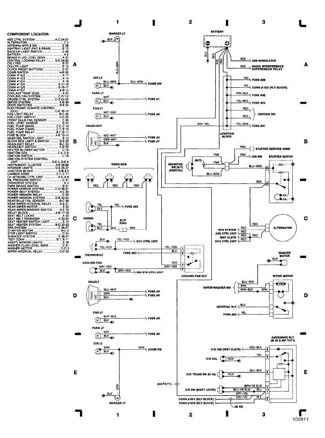
WIRING DIAGRAMS Fig. 2: Computer Engine Control (2.3L Turbo) 1988 Volvo 760
