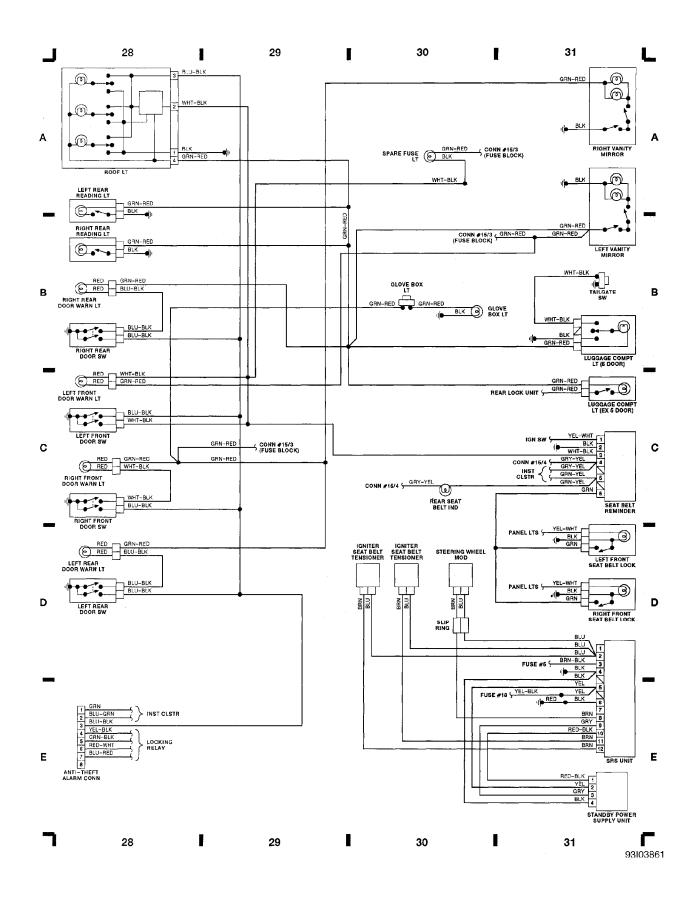
Fig. 9: Power Seat (W/Memory), Memory Control Unit (Grid 32-35)
