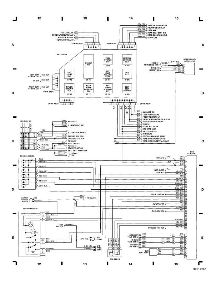
Fig. 5: Comb Sw, Pwr Window, Wiper/Washer, Headlt Sw (Grids 16-19)
